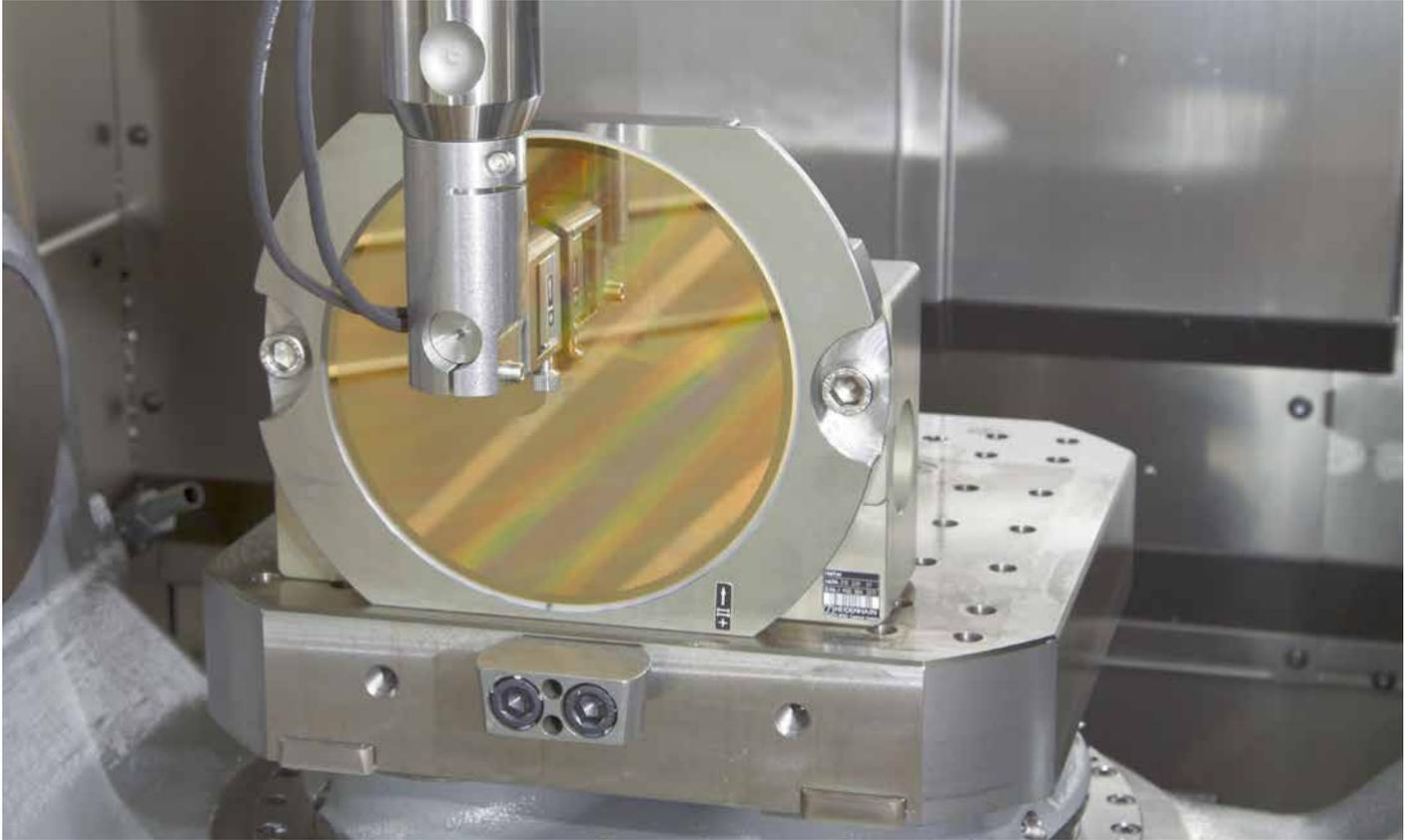
Figure 5: Measuring test setup with KGM 181 grid encoder
