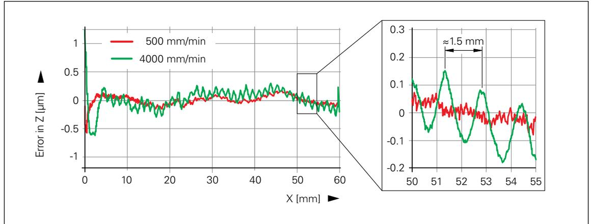
Figure 7: Measuring results with rotary encoder 2
