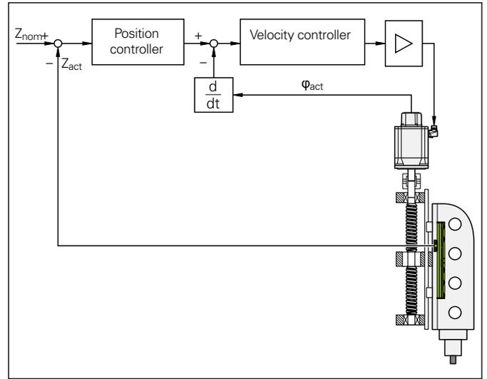
Figure 4: Schematic representation of a feed axis
