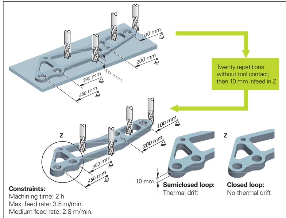
Figure 5 Manufacturing of the coupling lever
