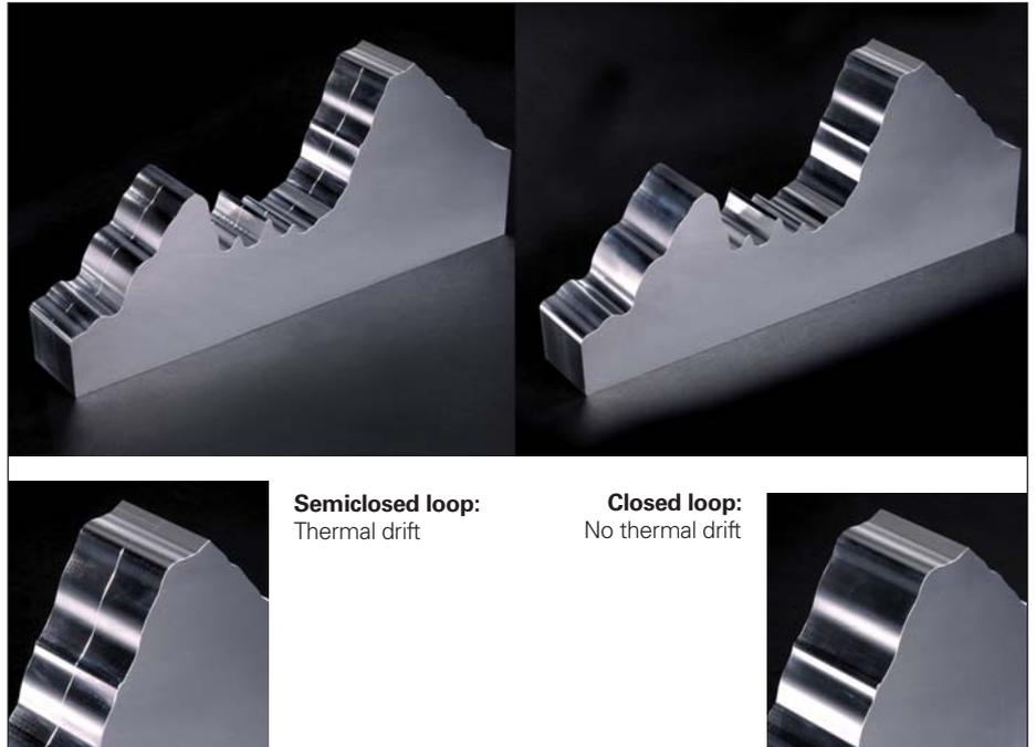
Figure 7 Watzmann profile with free-formed surfaces
