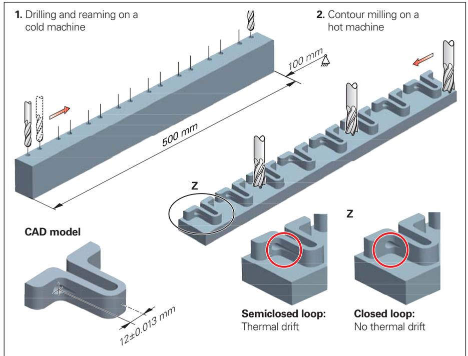
Figure 3 Effect of drive accuracy on the production of small parts
